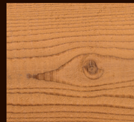
rough sawn: rustic, rough surface with a recognisable pattern from the cut of the band saw
