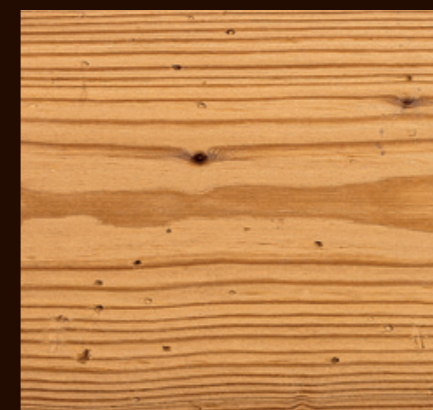
worm-finished: Imitation of worm- holes by a mechanical process
